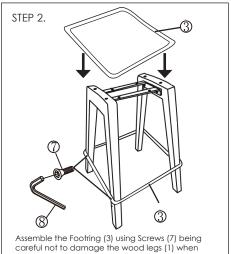
installing, DO NOT fully tighten Screws (7).
